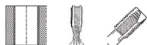
through holes up to 4 x D Chip removal (like picture) Form B with spiral point
