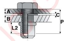
Closed Body End The screw length (P) for a closed blind rivet nut is linked to the material thickness of the riveted components (A+B) plus the head height or the gap size (C) in combination with the length of the internal thread L2.
