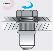
Tightening torque: The test assembly of the screw connection of a non-rotating component with a screw against the head of the blind rivet nut. While doing this, the load-bearing capacity of the nut thread is determined.
