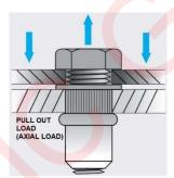
Pull out Load or sometimes referred as pus out. Load values given in the datasheets are only reference values.
