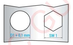
**Dimension of the drilling hole** - For cylindrical receiving holes, this dimension is referred to as the diameter D1 + 0.1 mm, and for hexagonal receiving holes - as the width across flats AF 1 (SW 1). Please see the recommended drilling hole dimension on the respective datasheet.
