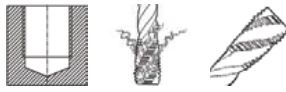
blind holes up to 3 x D Chip removal (like picture) Form C 40° spiral flute
